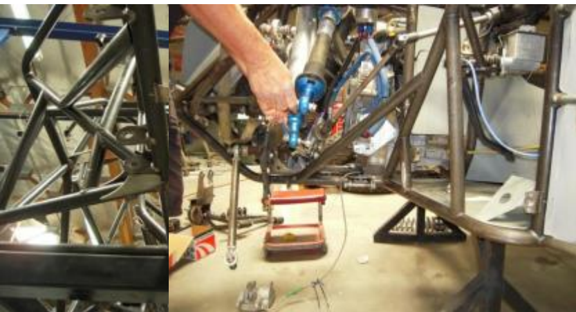
The bottom of the chassis with the new diagonal tube installed.
